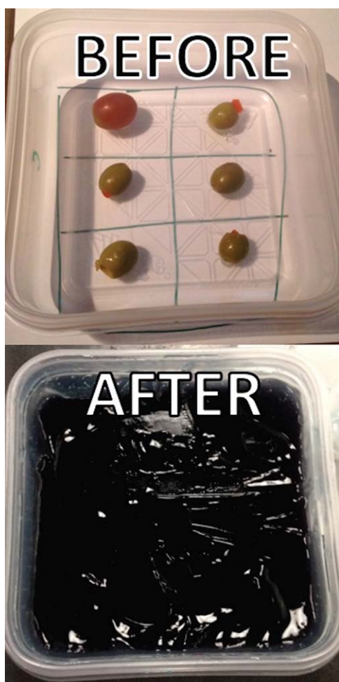
Figure 2. Large gelatin phantom containing grapes, olives, and pimento olives before and after the gelatin medium was added.
